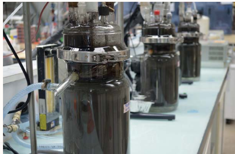
Multi-scale process development: : 2 L bioreactors. © BRGM
