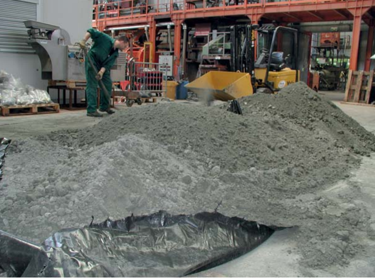
Preparation of 5 tonnes of mining waste from the copper industry for bioleaching recovery tests (France). © BRGM - Anne-Gwenaëlle Guézennec
