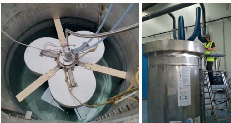
Multi-scale process development: "Pond bioleaching" pilot (2000 L.) in BRGM laboratories. © BRGM
