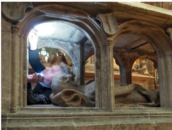
Sampling of alabaster from the tomb of the Hessian landgrave, William II (1515) in Marburg, Hesse, as a part of the Louvre II project (Marbug, Germany, 2018). © BRGM - Wolfram Kloppmann
