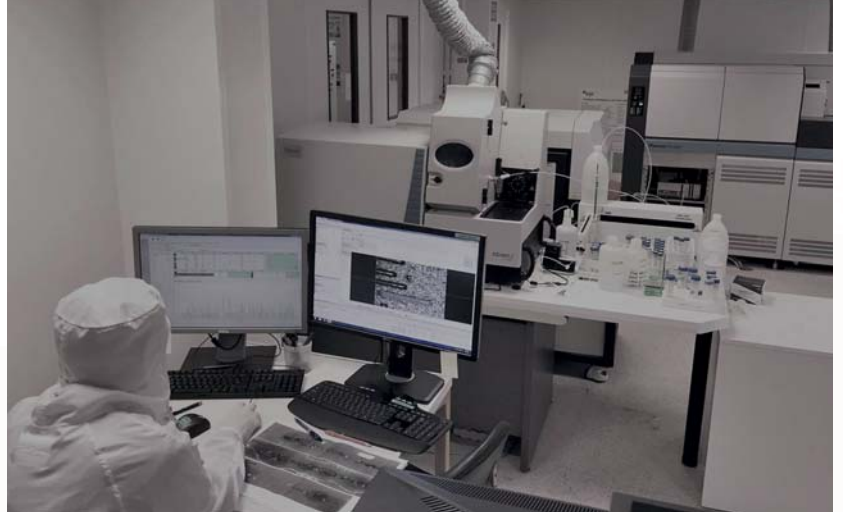
Elementary measurements by laser ablation ICP-MS and isotopic analysis using the NEPTUNE MC-ICPMS – BRGM laboratories in Orléans. © BRGM
