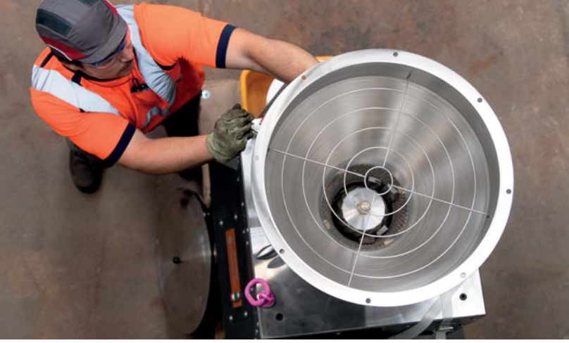
Notched gyratory crusher on BRGM's Plat'Inn platform (Loiret, 2020). © BRGM – Didier Depoorter
